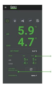
The Min/Max temperatures displayed are the lowest and highest recorded AIR and LOAD temperatures since the latest reset.
