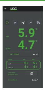
2 Both AIR and LOAD temperatures will be reset **NOTE:** After pressing RESET the Min/Max temperatures are stored in the controller for up to 3 months on FIFO bases.
