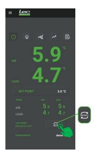
1 To reset the min & max temperatures simply press the reset button
