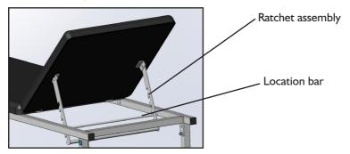
To lower the backrest, take the weight of the backrest with one hand and slightly lift. With the other hand disengage the ratchet assembly away from the location bar and lower the backrest.
