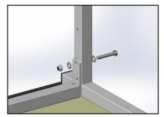
4. With the couch upside down, position one side of the leg onto the lug and location peg. With this in place gently ease the opposite leg outwards onto the second location peg.
