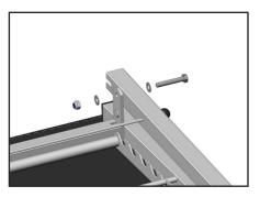
3. Carefully cut the cable ties holding the legs and ratchet support arm to the frame and remove the nuts, bolts and washers holding the legs in place. Keep these parts safe as they will be re-used later.
